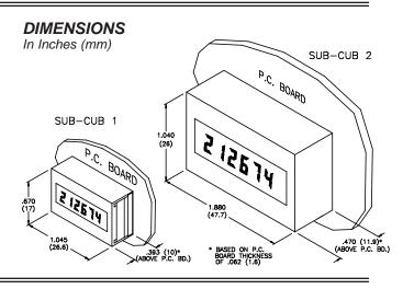
Note: All hole size tolerances ±0.003" (0.08 mm) All other tolerances ±0.005" (0.13 mm)
